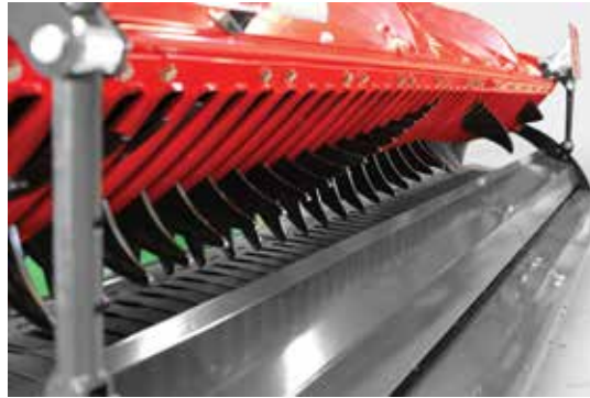
The finger rotor in combination with the pick-up ensures the perfect crop flow.
